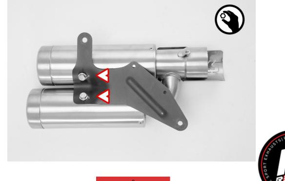
Mount the REMUS connection tube onto the serial header. Install the supplied additional bracket. Use the supplied screws and spacers.
