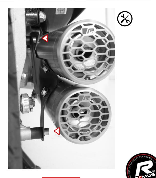
Align the REMUS sport exhaust and tighten the connections.
