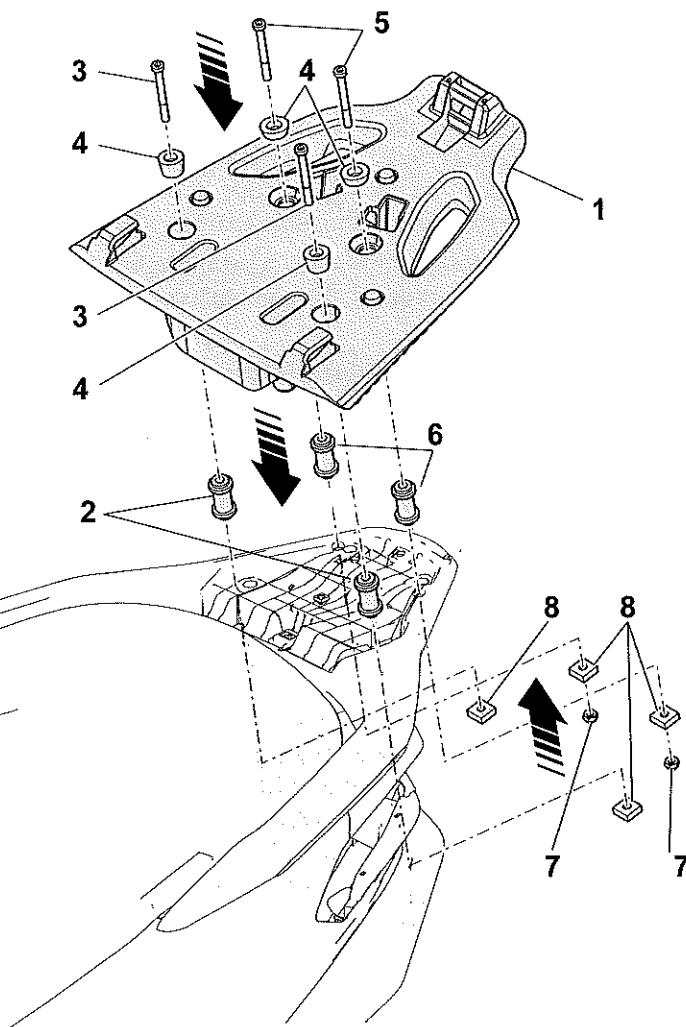
**GB** Position the top box plate 1 in correspondence with the holes on the luggage rack, taking care to insert the spacers 2 and 6 as shown in the figure.
