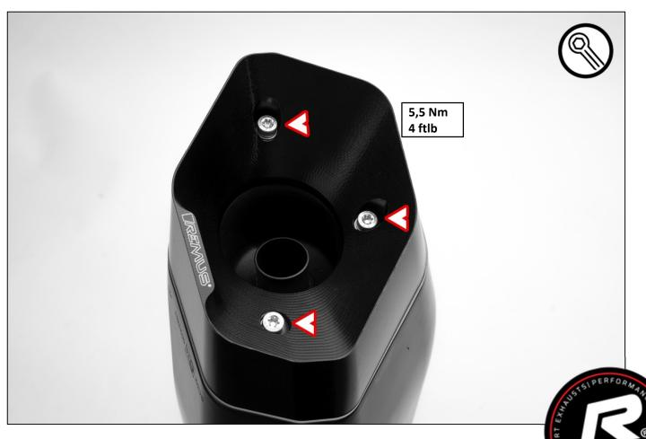
Install the supplied bracket onto the REMUS sport exhaust.
