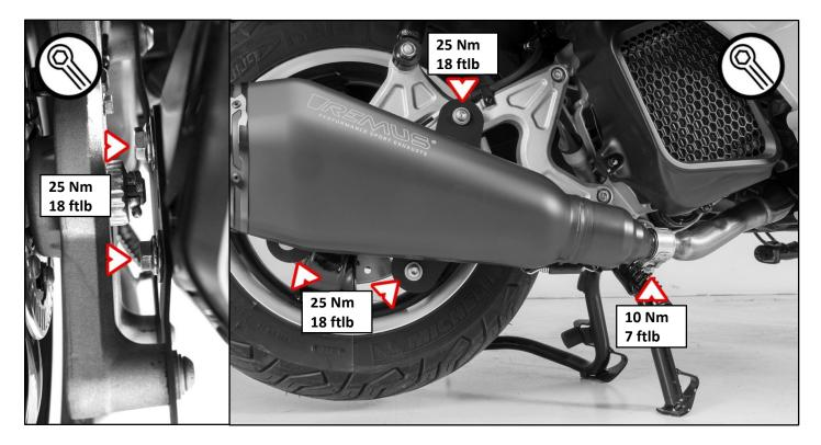
Tighten the screws of the stock header again.
