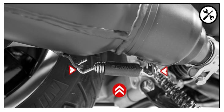
Align the REMUS sport exhaust and tighten the connections.
